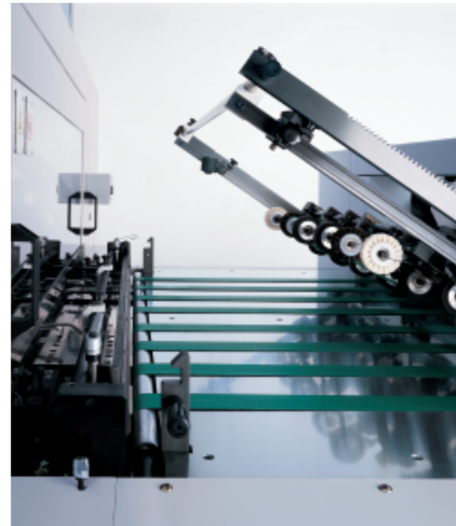
Central setting of the belt table rollers reduces makeready time and improves sheet travel. 1
